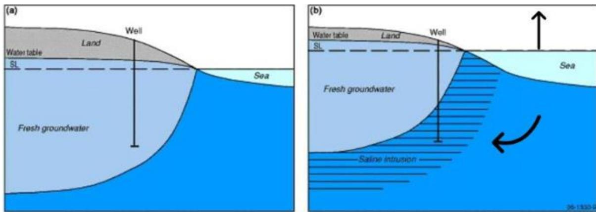
**Figure 6.** Salt water intrusion caused by sea level rise (Bergkamp *et al.*, 2018).
