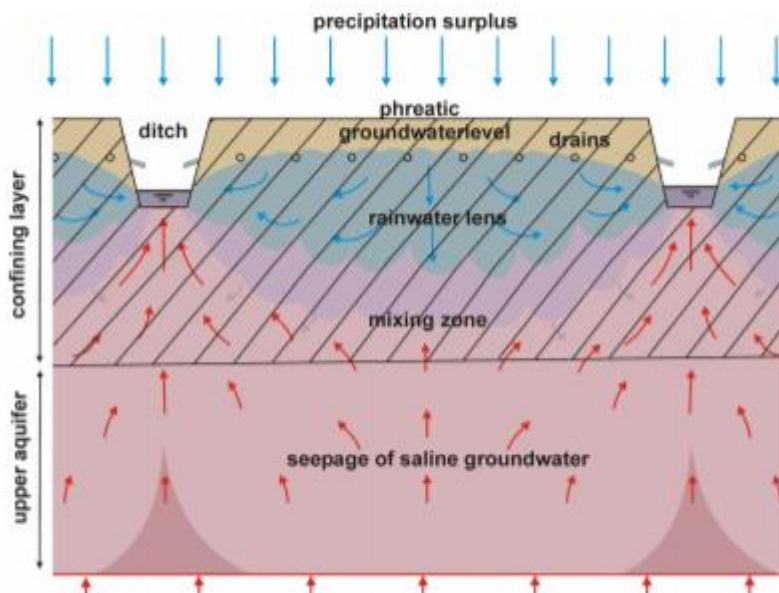
**Figure 4.** Conceptual visualisation of a shallow rainwater lens on top of saline groundwater seepage (De Louw *et al.*, 2011).
