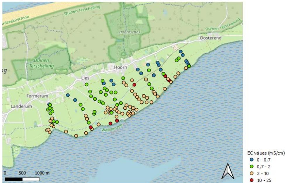
**Figure 9.** Surface water measurements from April categorized by EC values.
