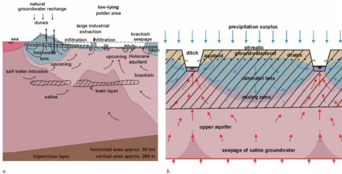
**Figure 7.** Salinization processes in the western Netherlands on a. regional; and b. local scale (Pauw *et al.*, 2012).
